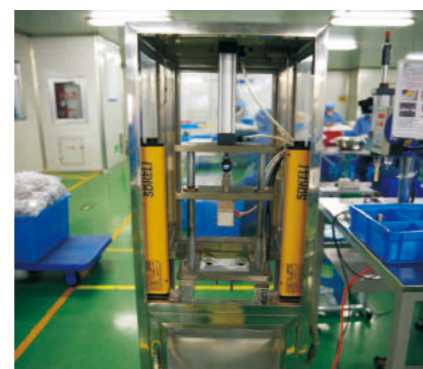
Heat welding 热焊接
